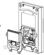
Make cables go through the back cover, connecting to the corresponding interfaces of the main board.
