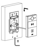
Insert the four wall-mounting screws on the device into the corresponding holes on the wall-mounting bracket, and then press down to slide the wall-mounting screws into the groove. Then use the Allen Wrench to tighten the device with two Allen screws.
