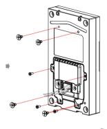
Fasten the back cover with four M2.5x6 screws, then fix four wall-mounting screws on the back of R20A-2.
